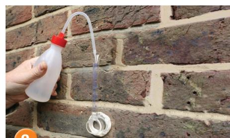
9 A Stormdry Gauge can be used to demonstrate the effectiveness of the treatment. The test should be carried out at least 28 days after applying Stormdry which allows the water absorption of the wall before and after treatment to be compared.
